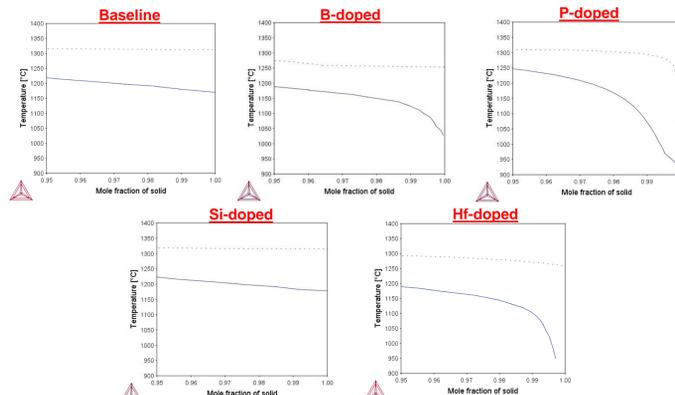
Figure 6: Scheil and Equilibrium solidification curves for the four altered chemistries.
