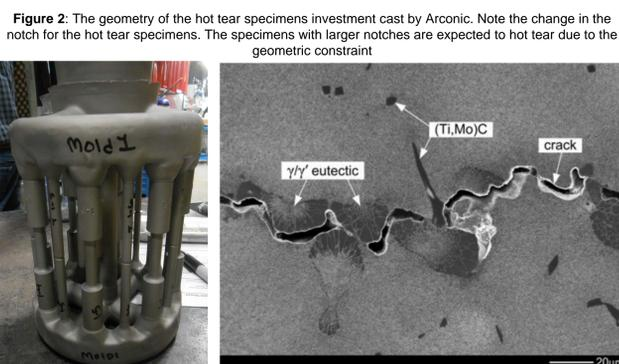
High temperature tensile testing at 2000 °F was utilized to replicate intergranular fracture during solidification. Thermo-Calc software was utilized to investigate solidification behavior with element additions. The samples were sectioned, mounted, etched, and analyzed via optical and SEM microscopy.
