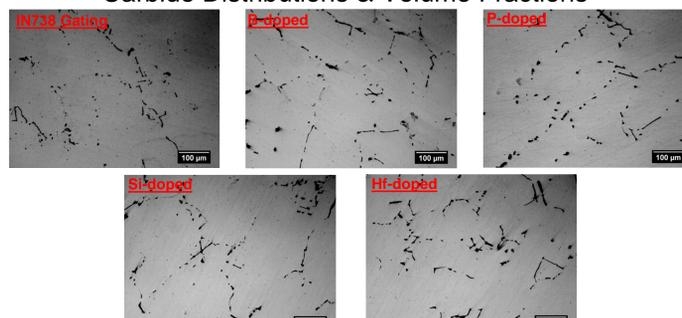
Figure 7: Unetched optical micrographs of undoped IN738 gating, B addition, P addition, Si addition, and Hf addition showing the carbides obtained from the chemistry slugs.
