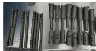
Figure 5: Hot tear specimens (left) and tensile bar specimens (right) after being broken out from the mold and sectioned.
